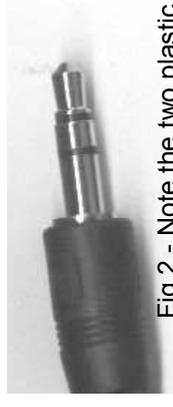
Fig 2 - Note the two plastic ring separation
